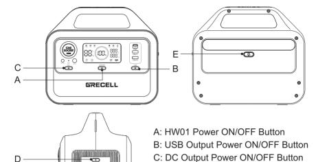
D: AC Output Power ON/OFF Button E: SOS Mode & LED Light Button
